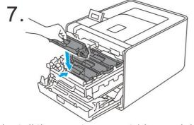
Install the new toner cartridge and drum unit assembly into the printer.
