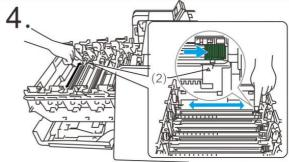
Gently slide the tab from right to left and left to right several times to clean the corona wire. Return the tab to the home position(2).
