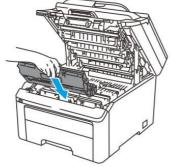
Install the new toner cartridge and drum unit assembly into the printer.
