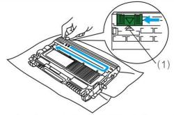
Gently slide the tab from right to left and left to right several times to clean the corona wire. Return the tab to the home position(1).
