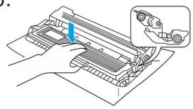
Put the new toner cartridge firmly into the drum unit until it locks into place.
