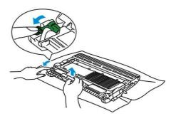
Push down the lock lever and take the used toner cartridge out of the drum unit.
