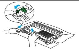
Push down the lock lever and take the used toner cartridge out of the drum unit.
