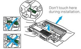
Unpack the drum and remove the black paper. Put the toner cartridge firmly into the new drum unit until it locks into place.
