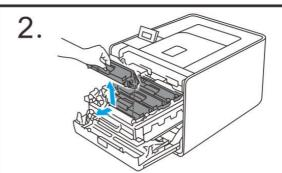
Pull out the drum unit and take out the used toner cartridge assembly.
