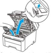
Open the front cover, take out the toner cartridge and drum unit assembly.
