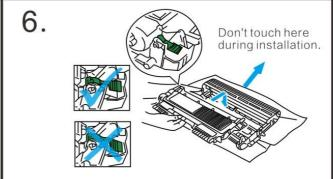
Insert the new toner cartridge into the drum unit until it locks into place.
