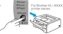
Reset the drum counter. With the front cover open, press and hold GO button for about 4 seconds until all the LEDs light up. Once all 4 LEDs are lit, release Go button.
