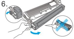
Remove the protective cover. Do not touch the developing roller.
