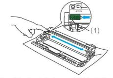
Gently slide the tab from right to left and left to right several times to clean the corona wire. Return the tab to the home position(1).
