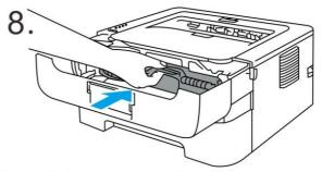
Install the toner cartridge and drum unit assembly into the printer.
