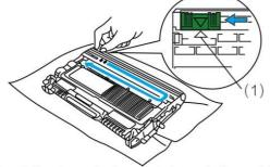
Gently slide the tab from right to left and left to right several times to clean the corona wire. Return the tab to the home position(1).
